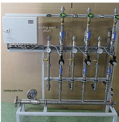
Cooling water control skid
